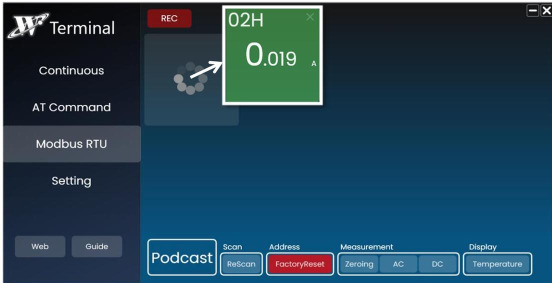
If already set up an address for sensor (**NOT 01H**), you can press **ReScan** button to show it on screen.
